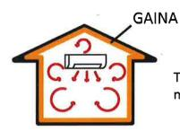
The temperature of the air and wall surfaces equalize, minimizing heat movement.
